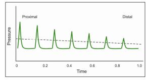
The LifePulse uses passive exhalation. Thus, airway pressure at endexpiration, PEEP, is constant throughout the lungs, as long as rate is set slow enough to avoid gas trapping.
